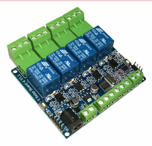
MODBUS RTU RELAY4/IN4 ... has 4 of RELAY ON/OFF and 4 of INPUT TTL(3.3V); it receives Commands through RS485 HALF DUPLEX. There is PROTOCOL as MODBUS RTU to command. The maximum distance of connecting signal is 1.2 kilometers long (separate Power Supply).
